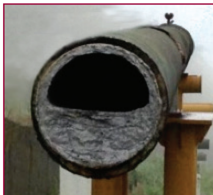
Untreated line with silica scale
