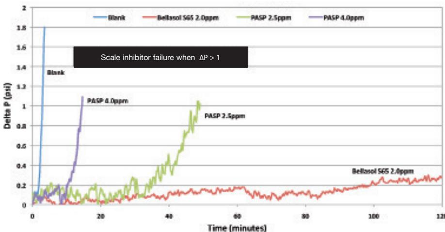
Figure 1. Brent water  $\text{CaCO}_3$  dynamic tube blocking test: dosed as solids.
