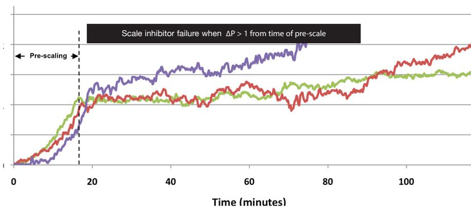
Figure 2.  $\text{BaSO}_4$  dynamic tube blocking test: dosed as solids.
