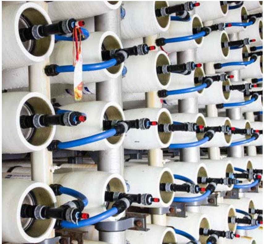
Novel: IDE Technologies has developed a cleaning system (DOHS) that eliminates chemical use in membrane cleaning
